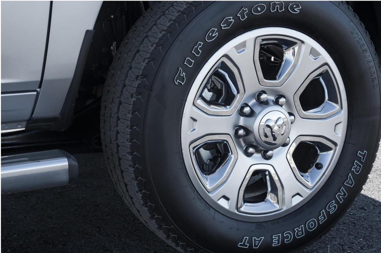
The customer must have a wheel with a center-hole or removable center cap. Dynatrac does not recommend modifying any part of the wheel. This will decrease the strength of the wheel and can lead to catastrophic failure. Most aftermarket wheels will have a removable center cap, but the customer must confirm before ordering. Dynatrac has confirmed the fitment of the following wheels:
