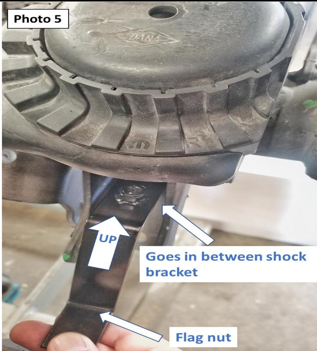
12. Install the front shock using the OEM hardware. Torque Upper bolt to 65 ft-lbs and lower bolt and nut to 65 ft-lbs. NOTE: Dynatrac does not recommend using power tools or air tools to tighten the shock hardware.
