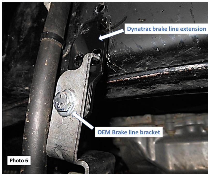
**ⓘ INFORMATION:** There is a Driver side and a Passenger side Dynatrac brake line extension. These extensions can only mount on the correct side.
