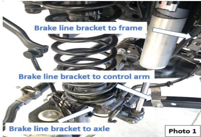
3. Cut and remove the clip from the axle vent hose that holds the brake line bracket
