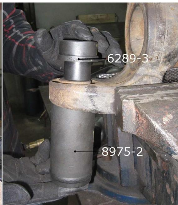
Figure 3, Pressing out OEM Lower Ball Joint
