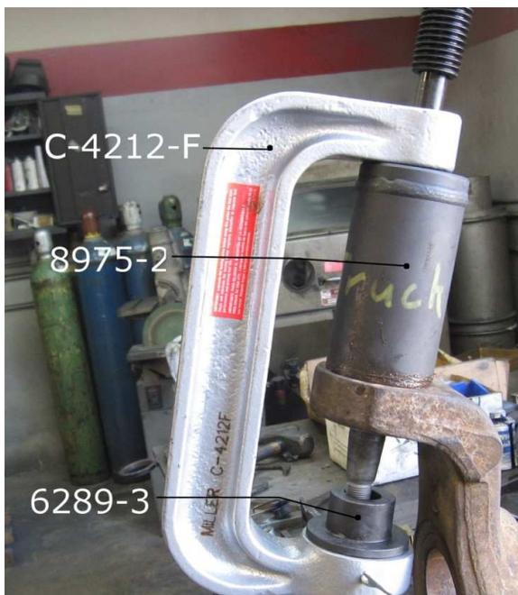
Figure 2, Pressing out Upper Ball Joint
