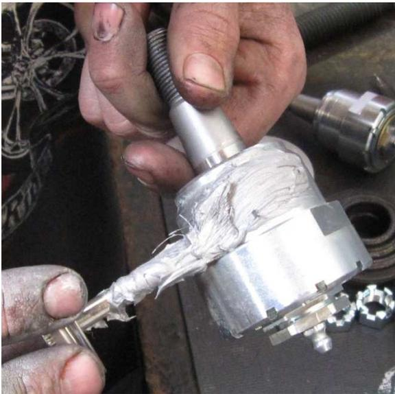
Figure 4, Applying Anti-Seize to ProSteer Body
