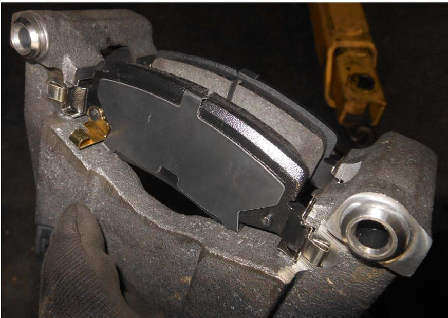
23. Once the caliper bracket is loaded, install it onto the backing plate using the factory fasteners. NOTE: Use thread locker on these bolts and torque to 77 ft lbs.
