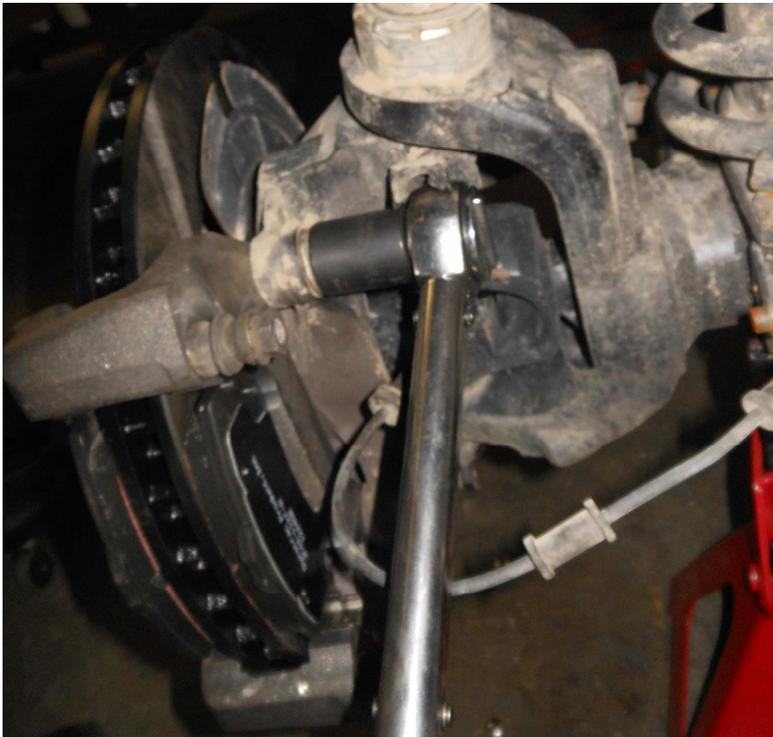
11. Now, remove and clean the caliper sliding pins from the factory caliper bracket. Fully clean and grease the pin and the inside of the boot before installing into the Dynatrac caliper bracket.
