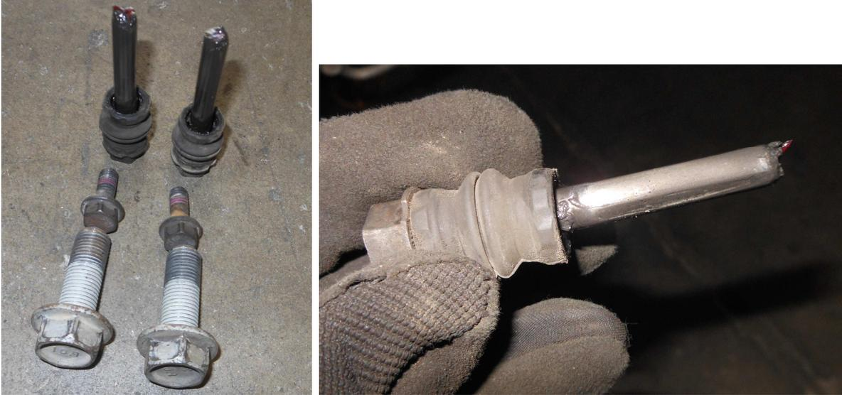
12. Once the pins are prepped and slid into the caliper bracket, the caliper can be installed onto the bracket. Take care when sliding the caliper over the new pads. Press in the caliper piston further if it will not fit over the new brake pad assembly.
