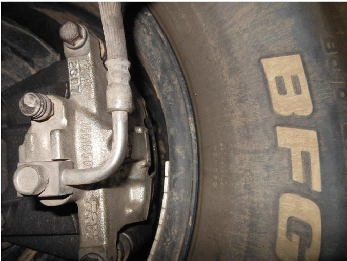
28. Once your wheels are back on the vehicle and torqued to the recommended 110 ft lbs., you should confirm that your brake fluid level is at the proper level. Test the brake pedal for pressure and make sure there are no leaks or loose bolts.
