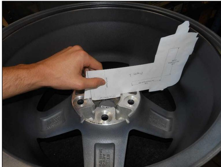
5. Take your completed profile and place it into the wheel. Make sure the wheel pilot is centering your cutout and that the cutout is resting on the wheel mounting surface.
