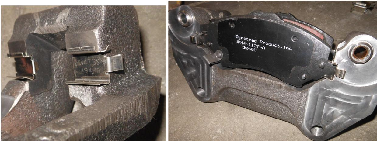
10. Fasten the Dynatrac Caliper Bracket to the Steering Knuckle with the factory bolts. Apply thread locker to the bolts and torque to 120 lb ft.
