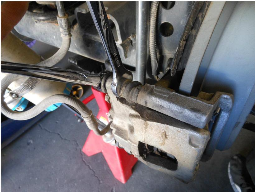
18. Next, the lower swaybar link bolt will have to be removed in order to reach the rear caliper bracket bolt.
