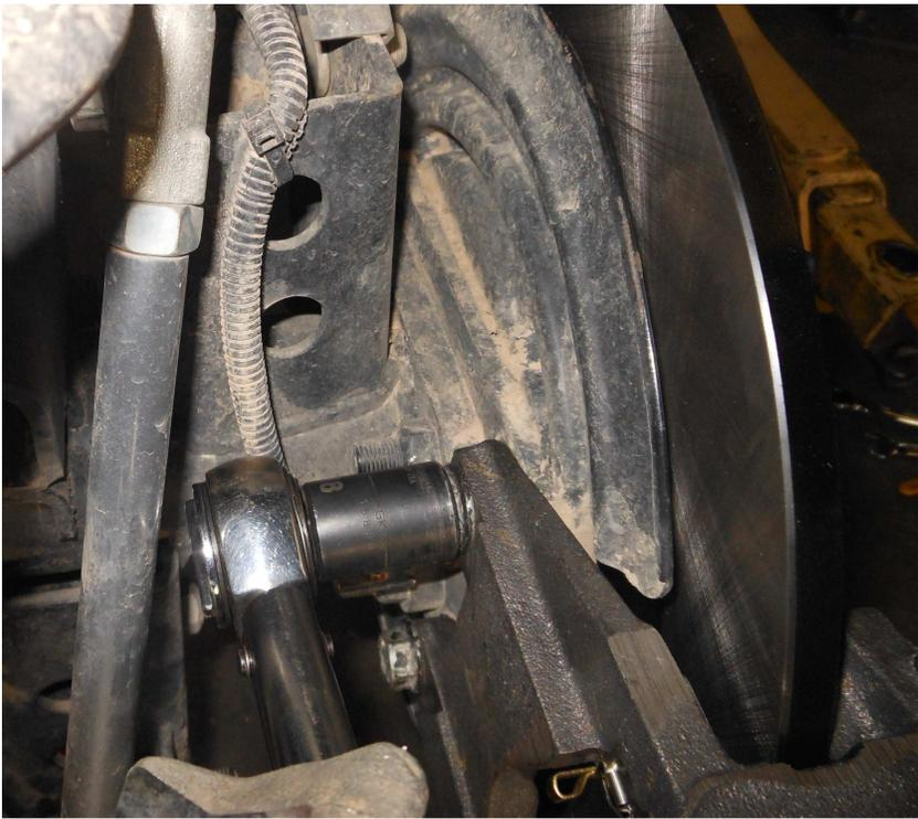
20. This is the best time to clean all the mating surfaces of the rotor and caliper, along any other dusty components.
