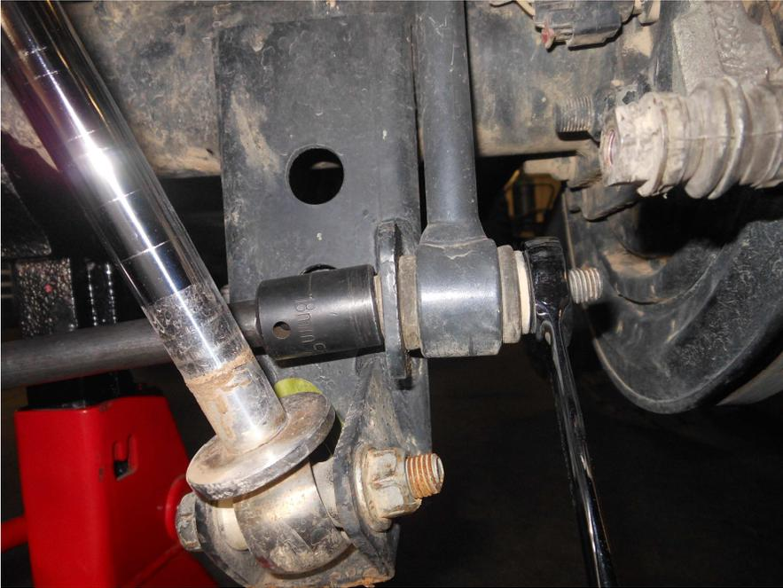
19. Now, uninstall the Stock Rear Caliper Bracket using an 18mm socket and set the hardware to the side for reuse.
