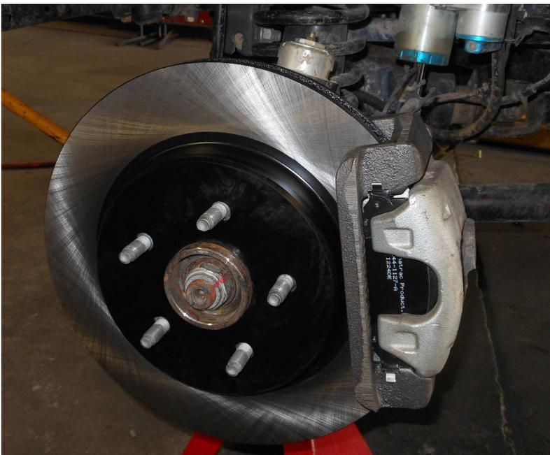
13. Apply thread locker and Torque the small caliper mounting bolts to 26 ft. lbs with a 13mm socket.
