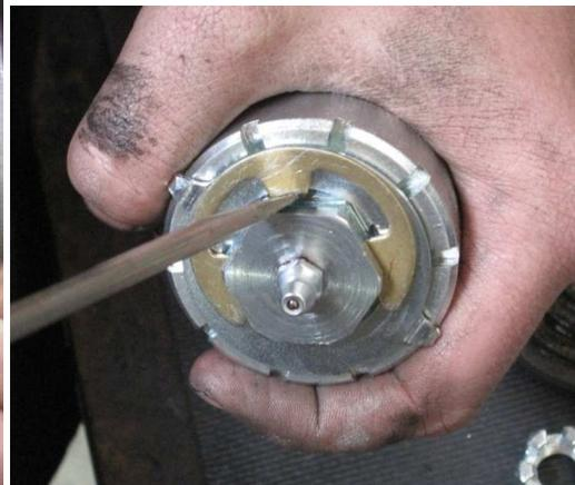
Figure 7, Removing E-Clip
