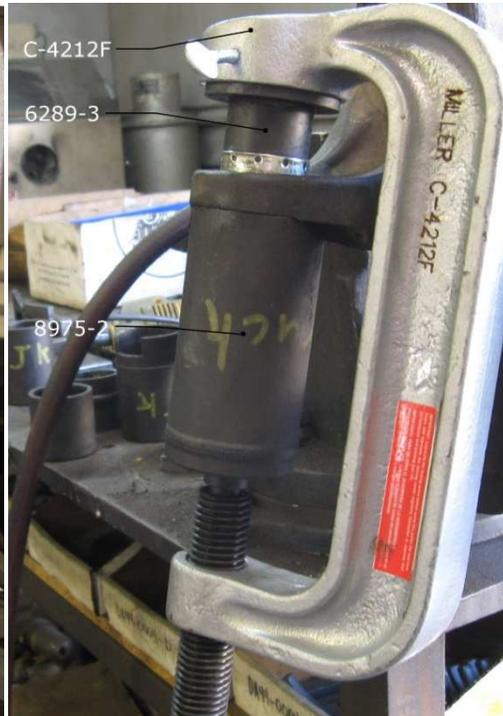
Figure 2, Lower Ball Joint Removal
