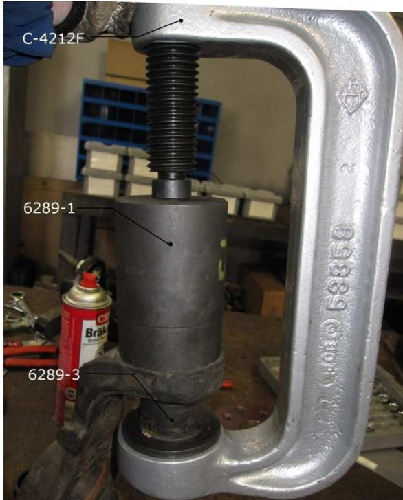
Figure 1, Upper Ball Joint Removal
