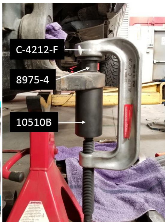
Figure 3. Pressing out OEM Lower Ball Joint
