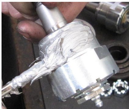
Figure 5. Applying Anti-Seize to Ball Joint Body
