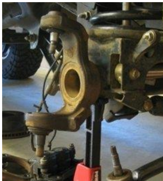
Figure 1. End Forging with OEM ball joints
