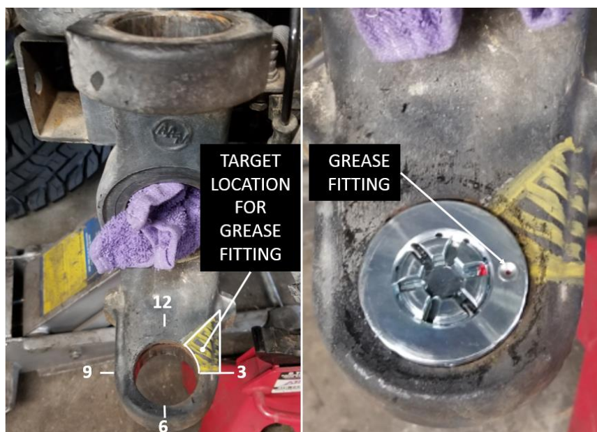
Figure 4. Driver Side Lower Ball Joint grease fitting orientation
