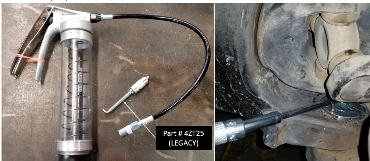
Figure 12. Lower Ball Joint grease gun needlepoint adapter
