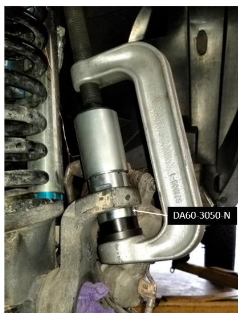
Figure 10. Installing Dynatrac Upper Ball Joint, second half
