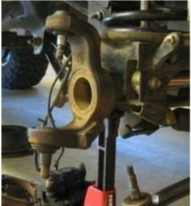
Figure 1, End Forging With OEM ball joints
