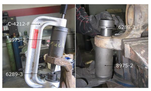
Figure 2, Pressing out Upper Ball Joint
