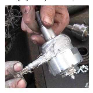
Figure 4, Applying Anti-Seize to ProSteer Body
