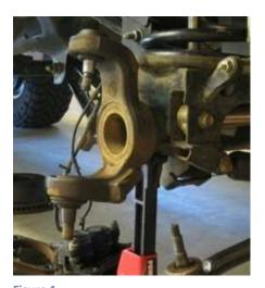
II. Disassembly of Upper Ball Joint
