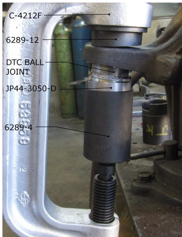
Figure 4, Installation of Lower Ball Joint
